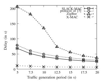
Figure 9. End-to-end delay of data packets as a function of the traffic generation period, for a duty-cycle of 1%, and for several protocols.
