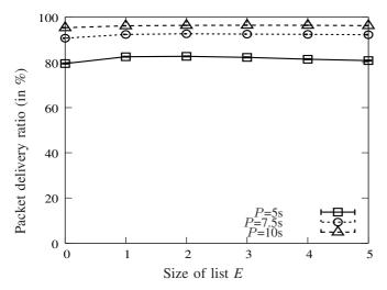
Figure 6. Impact of the size of list E of SLACK-MAC on the packet delivery ratio, with |R|=2|E| and a duty-cycle of 1%, where P is the traffic generation period.
