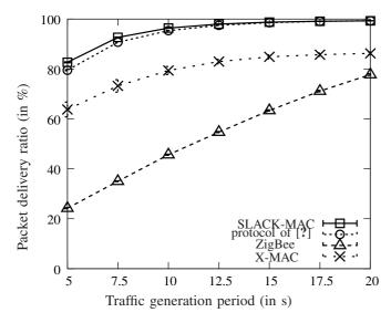
Figure 8. Packet delivery ratio as a function of the traffic generation period, for a duty-cycle of 1%, and for several protocols.
