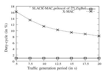
Figure 10. Duty-cycle (which is an approximation of the consumed energy) as a function of the traffic generation period, for a duty-cycle of 1%, and for several protocols.
