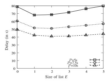
Figure 7. Impact of the size of list E of SLACK-MAC on the end-to-end delay, with |R|=2|E| and a duty-cycle of 1%, , where P is the traffic generation period.
