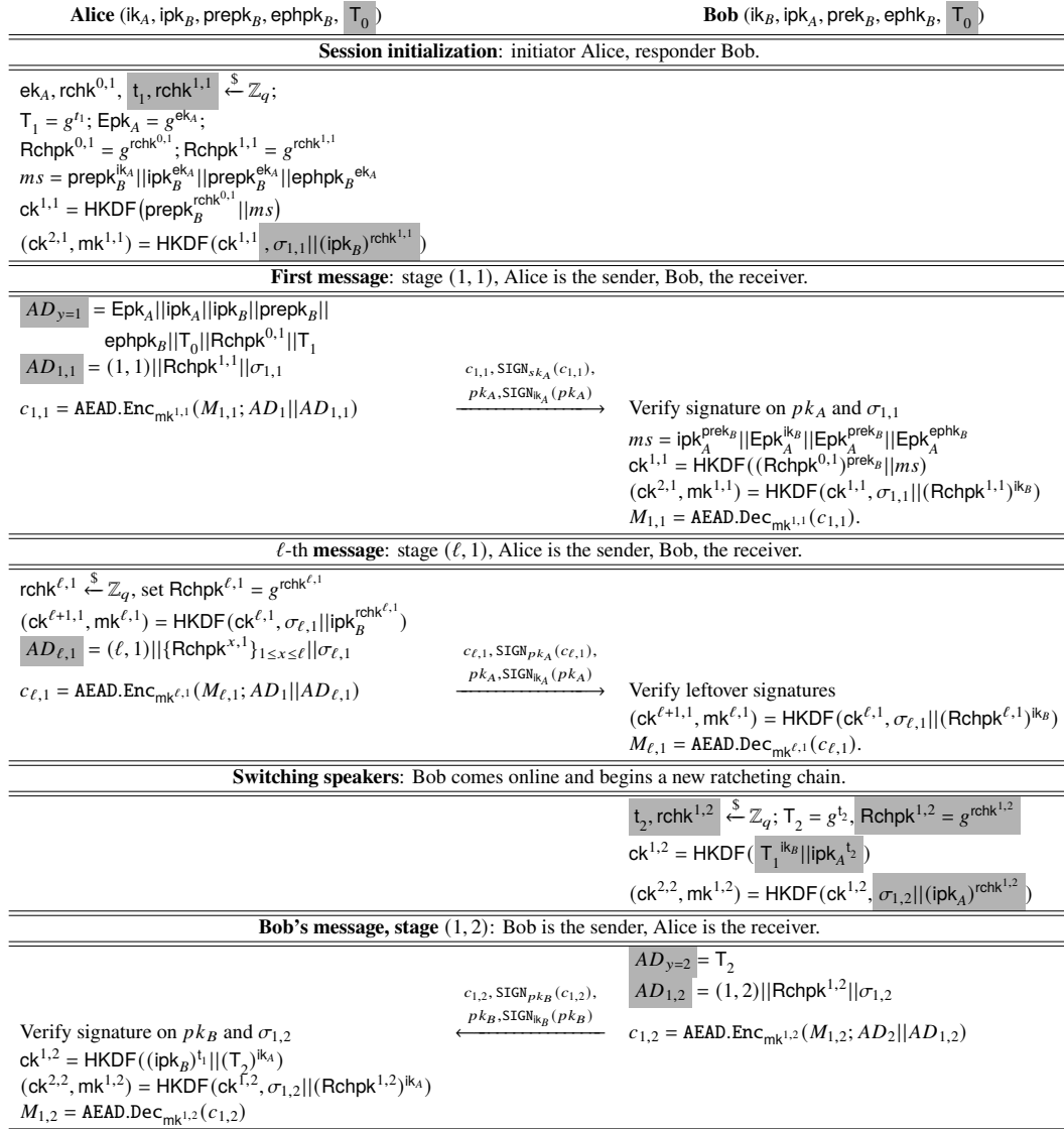
Figure 2.5 MARSHAL protocol execution between Alice and Bob for the first few stages. The grey boxes indicate modifications with respect to Signal protocol [CGCD + 17]. The transmitted data is also different but not in grey for more clarity.
