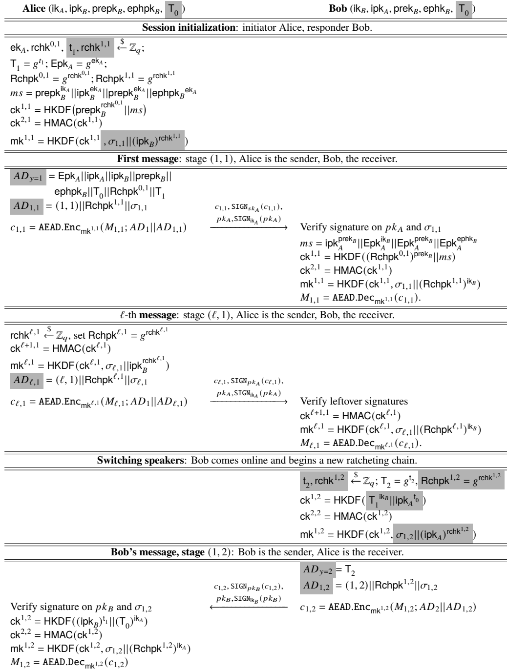
Figure 2.17 SAMURAI protocol execution between Alice and Bob for the first few stages. The grey boxes indicate modifications with respect to Signal protocol [CGCD + 17]. The transmitted data is also different and not in grey for more clarity.
